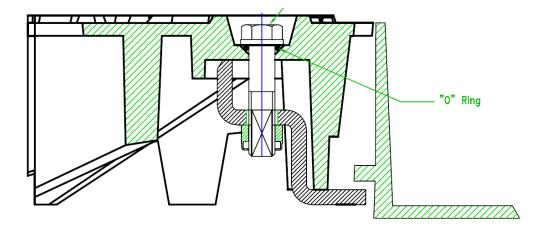
Lock configuration - cross section through cover section and frame Appropriate PPE should be worn at all times
