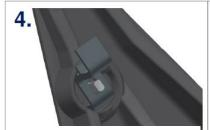
Place the locking bracket onto the bolt, correctly seating the squared-off shank of the bolt into the rectangular slot with the bracket tongue protruding over the cover rim as
