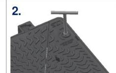
The lock is operated by using a 22mm socket drive as a key. Turning through 900 to the open position and closed positions as indicated on the primary cover section.
