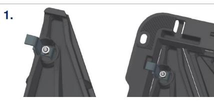
The above shows how the locking bracket swivels to engage underneath the cover section onto a retaining feature within the frame
